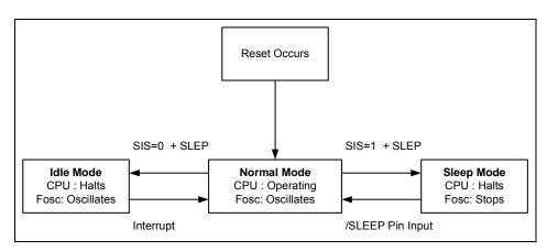
Fig. 5-4 Operation Mode and Switching
